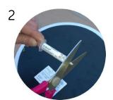
Cut off the nozzle of the polymer adhesive applicator (included).
